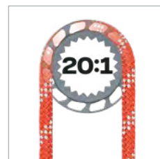
Ratchet block holding power
