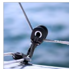
Cheek plates twist to open block
