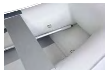
P270SH Aluminium seat, two bow lifting eyebolts for davits.
