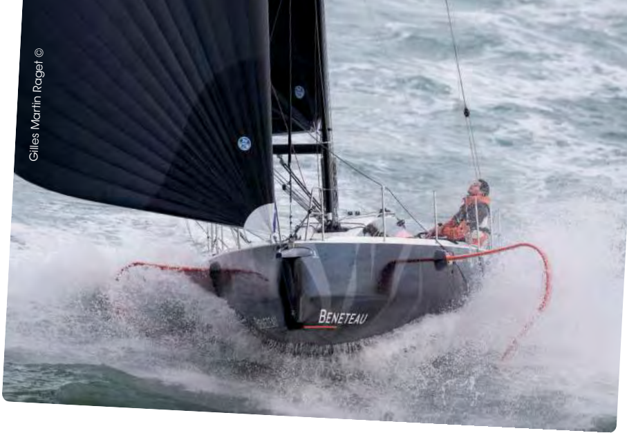
Beneteau Figaro 3, the world's first production foiling monohull.
