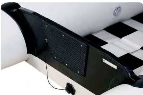
Painted wood transom features a PVC gunnel on upper rim to prevent water ingress.
