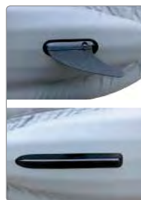
Rudder plank and directional band.
