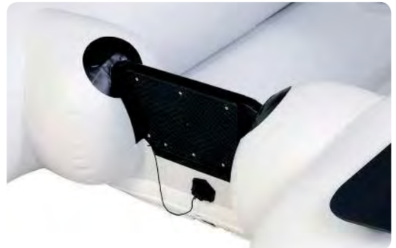
Rigid inflatable tube extensions on both sides of the transom contribute to a lightweight tender, more compact to stow.
