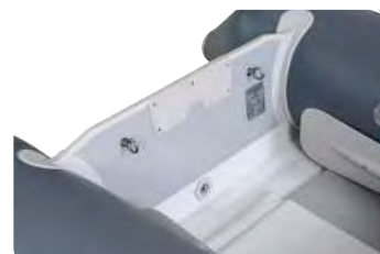
P270SH Paddles stowed and secured inside the boat. Two rear lifting eyebolts for davits.
