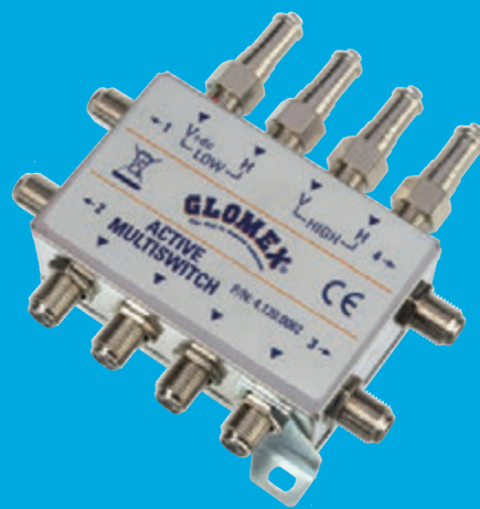
V9191 ACTIVE MULTISWITCH 4X4 - FOR MULTI OUTPUT SATELLITE ANTENNAS
