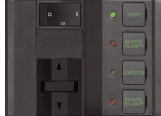
Circuit Breaker Source Selection
